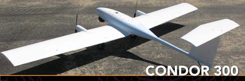
Condor 300's payload tray can accommodate a variety of commercial payloads including Cloud Cap Technology' TASE and TASE Duo gyrostabilized cameras.
